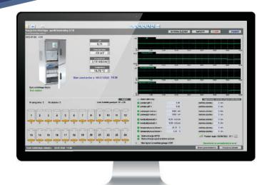
The MSX water and wastewater sampling and monitoring station MSX manufactured by our company can be integrated with transmitters for continuous measurement of pH, conductivity, dissolved oxygen, redox potential, COD, and temperature.
